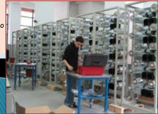
Routine and Insulation Test of Compenzeztion Board Supervised by Siemens Engineer in Our Workshop.
