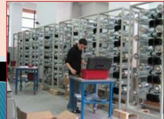
Siemens 8PU 152 Compenszation Panel Electromontage Manufacturing
