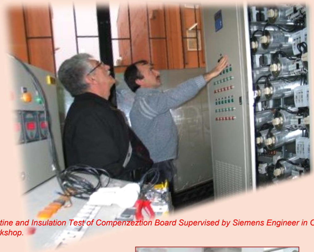
Siemens 8PU 152 Compenszation Panel Electromontage Manufacturing
